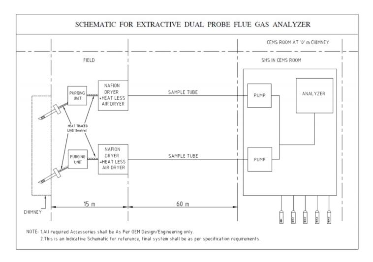
Note 12: Location of probe is at 35mts & analyzer is at '0'm of chimney. 15mts of HTL to be considered till Permapure Dryer in case of Extractive system. Permapure Dryer & Primary SHS shall be placed near probe at 35m elevation.
